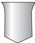
This face is used mainly on thicker material to reduce tonnage.
