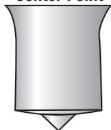
This standard face includes a center point for alignment and a crown face to reduce chipping of the cutting edge in heavy punching applications.
