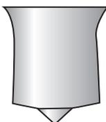
This face is also used on thicker material to reduce tonnage but has a center point for alignment.
