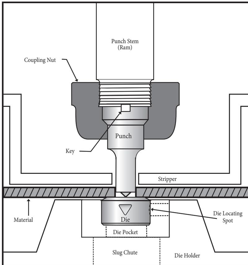
**Punch:** The male (usually upper) portion of a punching set-up determines the hole size. The hole (punch) must be slightly larger than the bolt or rod passing through it.
