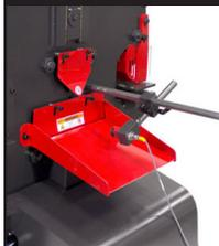
Adjustable proximity switch automates production when cutting repeatable lengths
