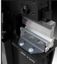
Controlled, repeatable bends in 1/4" thick mild steel
