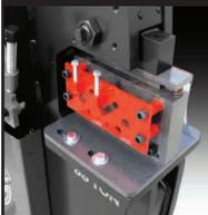
Combined Flat Bar, Angle, and Rod Shear for mild steel
