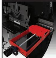
A positive stop attachment that is used to ensure accurate bending
